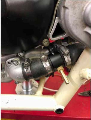
Once completed make sure to secure all pipes with supplied tie wraps in a way to avoid damage as pictured below.
